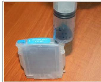
**3. ONCE THE CARTRIDGE ABOUT ¾ FULL OF INK, IT IS CRUCIAL TO INSERT AN EMPTY SYRINGE WITHOUT A NEEDLE INTO THE INK PORT OF THE CARTRIDGE, PRESSING ON IT AND MAKING SURE YOU HAVE A GOOD SEAL.**
